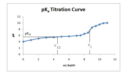
The equivalence point  $(V_1)$ , which is point where the curve is the steepest, and the half-equivalence point  $(V_{1/2})$  of the titration. Using the half-equivalence point the pK<sub>a</sub> of the unknown acid, and from the volume of base added at the equivalence point, the equivalent weight of the acid can be calculated. A list of all the possible acids for you to consider along with the pK<sub>a</sub> value for each of the acids will be provided by your instructor.
